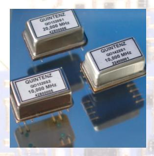
These miniature OCXO's in surface mounted technology reach stability values which can only be achieved with a basically bigger design by other manufactures.
